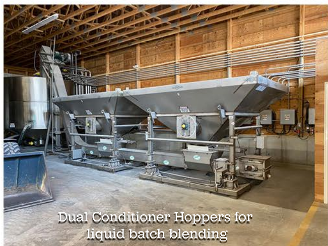
Dual 10-ton Rotary Blenders with batching hoppers
